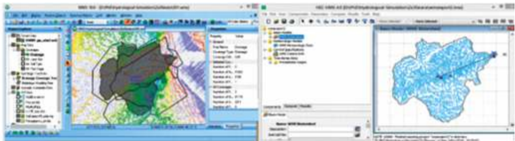
Figure 7 the hydrological model was built in WMS (left) then it was exported to be run in HEC-HMS (right)
